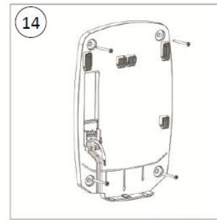
Screw the Plug-in base to the wall(x4)
