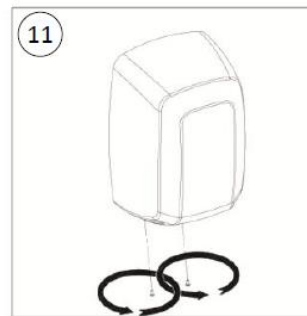
Screw the cover fixing screws (x2) Your dryer is now ready to be used on a Plug-in base
